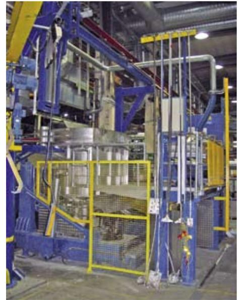
Fig. 6: Channel-type melting furnaces of 2-tonne capacity
