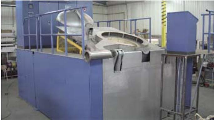
**Fig. 9: Special coreless induction furnace for producing an aluminium alloy with higher tin amounts**
