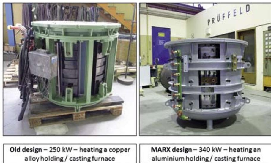
Fig. 4: Coreless inductor designs
