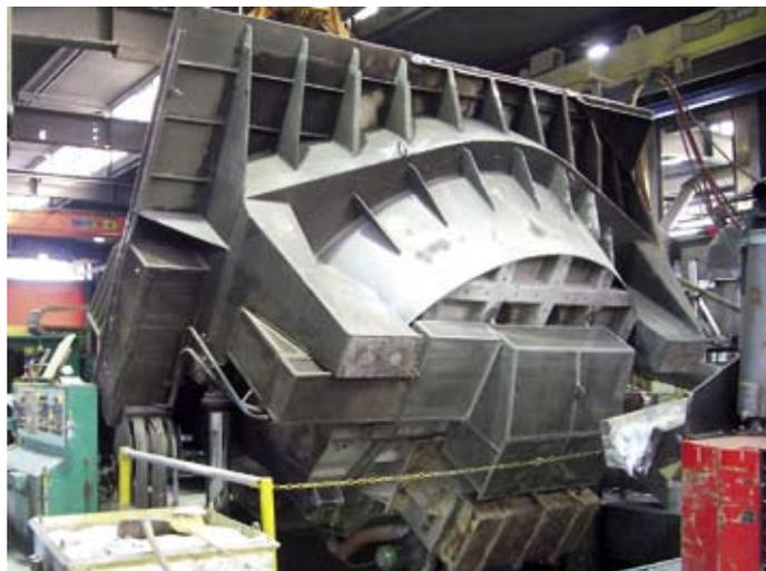
Fig. 7: Channel-type holding furnace
