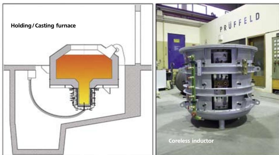
Fig. 3: Different types of induction furnaces – Furnace heated by coreless inductor
